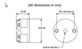
The SEM310 is mounted using two holes, on standard 33 mm fixing centres and will fit a DIN standard termination head. The SEM310 must be installed with adequate protection from moisture and corrosive atmospheres. Refer to conditions for use section of this user guide for information on enclosure IP rating.
